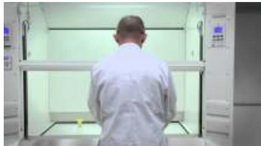
The reason for the inclusion of this is to reduce the face velocity under the sash, as the sash is lowered. (A smaller open sash area for a constant volume extract will result in a higher face velocity.) It is not practical to have a bypass opening, which is equal to the sash opening at 500mm, due to constraints on the height of the fume cupboard. Therefore, most fume cupboards will produce a face velocity of between 1.0 to 1.5 m/sec in the closed position.
